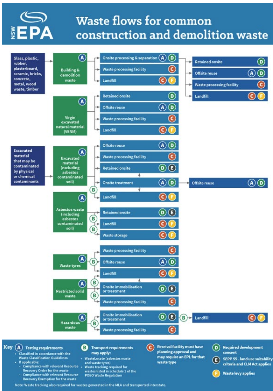
Figure 4-1: EPA Waste Flow Considerations During Construction and Demolition (Source: (EPA, 2020))
